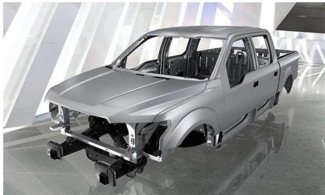
Aluminium panels for Ford's F150 manufactured by Novelis<sup>7</sup>
