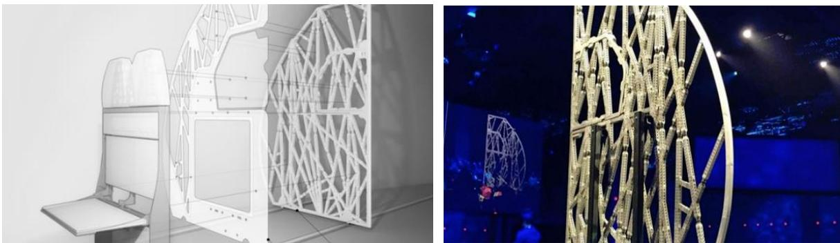
3D Printed Scalmalloy® RP partition and Aleris creep formed AlMgSc part<sup>3</sup>
